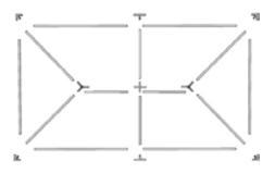
2. Start assembling the frame by inserting and pinning the Hip Rafters into the Center Crown(s). If assembling a rectangular frame insert and pin the appropriate Spreader into the Center Crown and continue to the next Ridge Top T or Center Crown. Insert and pin Rafters into the Crowns and Ridge Top T's. Insert and pin all Corner Fittings and Side T Joints to the bottom of the Hip Rafters and Rafters.
